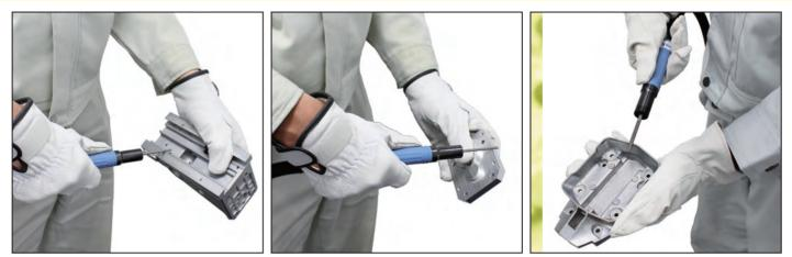
Best suited for deburring of die-cast aluminum products and machined parts.
