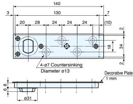
When using for the smoke ventilations or air intake doors (automatic opening), use the Auto-Hinge left and right opposite. Also use the U-2NH receptive base.
