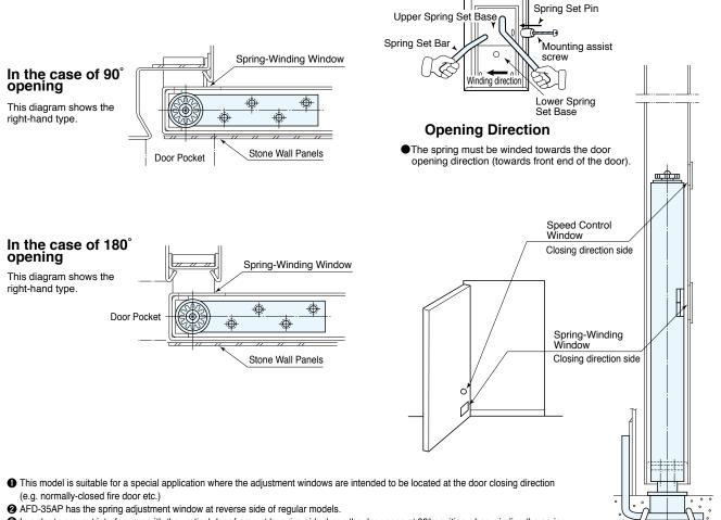
In order to prevent interference with the vertical door frame at hanging side, keep the door open at 90° position when winding the spring.
