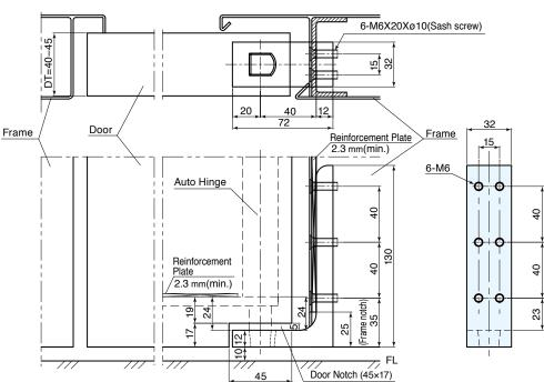
• Applicable wicket door size: 130 kg or less in weight, 40-45 mm in door thickness. (Compatible with A-8KH to 14H, AFD-8KH to 14H) P For NU-3LA, use a reinforcement steel plate of at least 3.2 mm thick and 200 mm long. For Auto-Hinge, use a reinforcement steel plate of at least 2.3 mm thick and 200 mm long.
