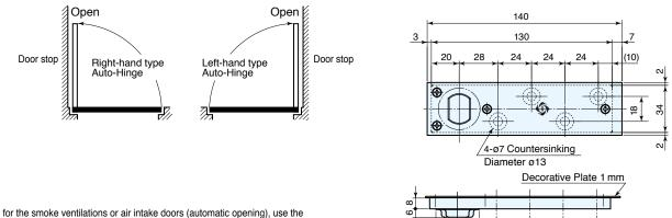
When using for the smoke ventilations or air intake doors (automatic opening), use the Auto-Hinge left and right opposite. Also use the U-2NH receptive base.
