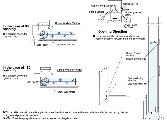
(3) In order to prevent interference with the vertical door frame at hanging side, keep the door open at 90° position when winding the spring.
