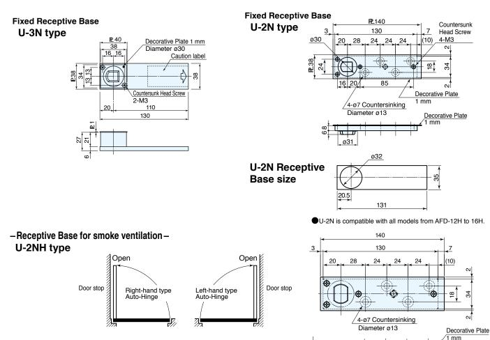
When using for the smoke ventilations or air intake doors (automatic opening), use the Auto-Hinge left and right opposite. Also use the U-2NH receptive base.
