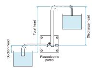
The discharge pressure of the bimorph pump is the measurement value when the suction head is zero, so the discharge pressure = the total head.
