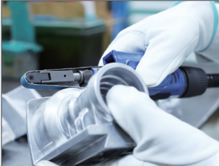
Deburring of die cast parts
