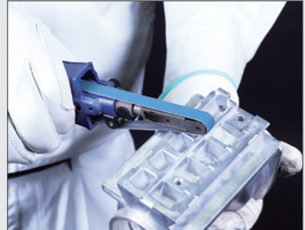
Chamfering of straight parts
