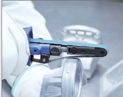
Detail finishing of aluminum material
