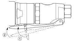
2 Hold the tool and while pressing the Lock Lever (1), press the Throttle Lever (2) The tool starts.
