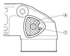
3 Perform a trial run and wipe off extra grease that seeps out Attach a Connecting Hose to the Cupla of the tool and operate the tool. At that time, grease may scatter from the exhaust part and Grease Inlet, so use with care. Stop the tool in a few seconds and always detach the tool from the Connecting Hose, then wipe off any grease that seeps from the periphery of the Spindle.
